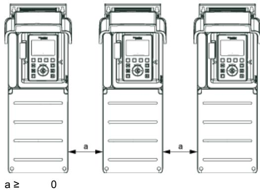
Mounting Type B: Side by Side IP20
